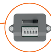
DIP switch inside the box, lower inventory
